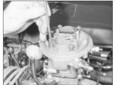
16.26 Removing a Torx through-bolt - 1.1 and 1.3 litre HCS engines
