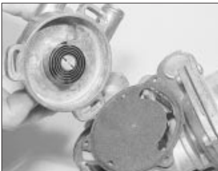
11.5 Removing the automatic choke bi-metal housing
