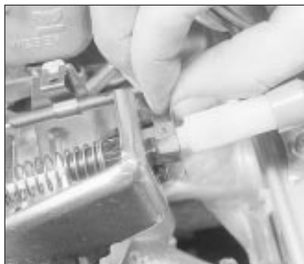
7.11a Prise out the throttle cable retaining clip . . .
